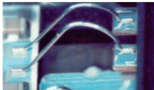
Figure 2: Connection of substrate to housing path
