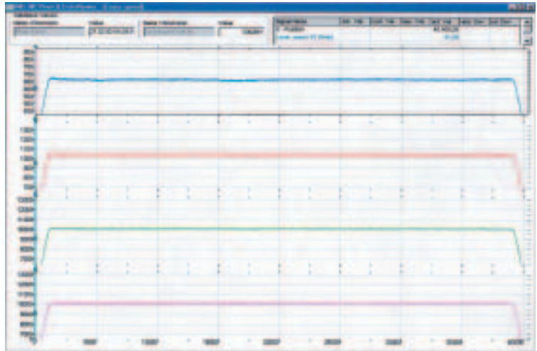
Figure 3: Strip velocity of four Polytec LSVs integrated in IMS C-frames (in the 5-stand tandem mill at USS-Posco in Pittsburg, California)
