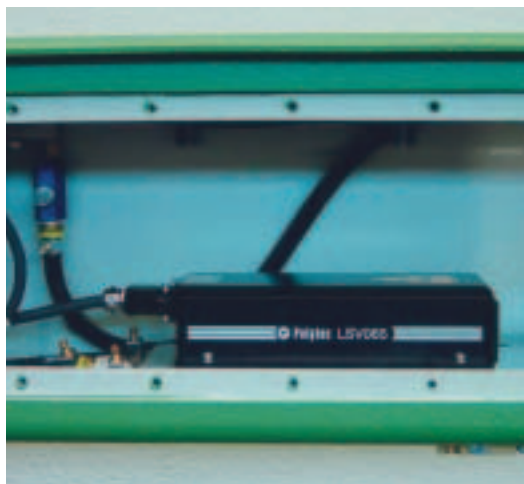
Figure 1: IMS C-frame with integrated Polytec LSV
