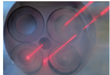
Fig. 3: Measurement and reference laser beams of the vibrometer.
