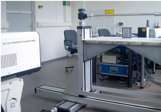
2 Laboratory setup: Excitation laser with scanner (right, back-ground); positioning stage with sample (center); Scanning Laser-Vibrometer (left, foreground).
