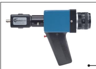
With the 7215-202 accessory, the 7215 can also be attached to CCTV cameras extending their spectral range to 1.5µm.
