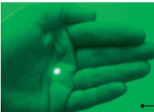
The 7215 is ideal for locating and aligning near-infrared laser beams and for identifying stray IR reflections that may otherwise go undetected.
