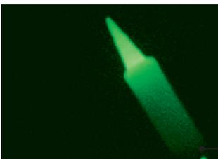
As a thermal imager, the 7215 can be used to view the radiation from objects hotter than about 600°C (such as the soldering iron shown).
