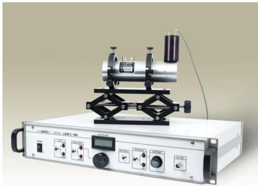
The LASS-II (Laser Amplitude Stabilization System) is an electro-optic feedback loop designed to reduce amplitude variations commonly associated with most gas lasers. This system is capable of significantly enhancing the signal/noise ratio of the laser over a much broader bandwidth than typical optically coupled current modulation of the plasma tube. Both an internal and external reference input is provided, allowing analog programming of the laser throughput. This is particularly convenient for
