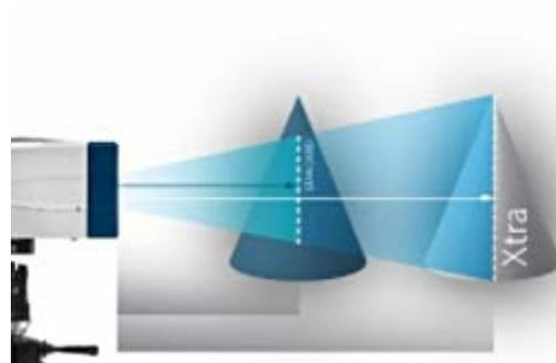
responsible for the signal-to-noise ratio of the measurement, the maximum achievable stand-off distance and therefore the size of the scanned area.
