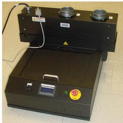
Users control the SPEED, STEP, and POSITION through the control panel on the Linear Stage. The Mode and operation of the Linear Stage is controlled through the X-1100 touchscreen user interface.
