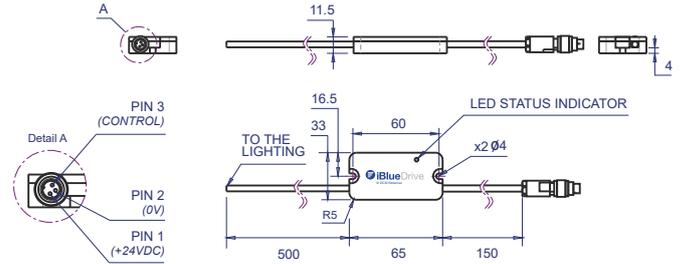
**WARNING!** In continuous and powered mode, clamp driver to a metal surface for heat dissipation. In Strobe mode is not required, but recommended.
