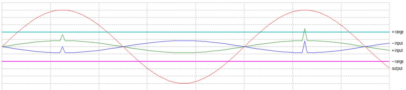
figure 2 common-mode removed at the input-stage: input-signal + disturbance can be above the input-voltage-range
