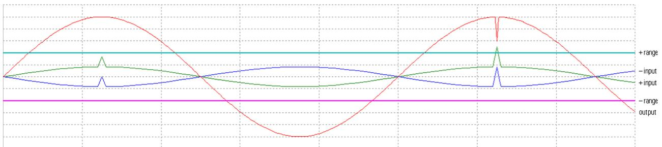
figure 1 common-mode removed after the input-stage: input-signal + disturbance must be within the input-voltage-range
