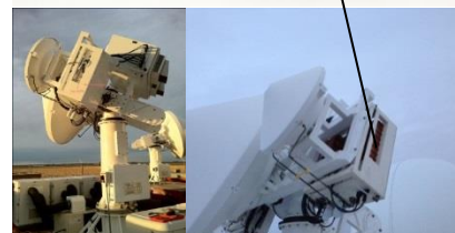
High Power Ka-band Amplifier for D3R and the Radar at CHILL facility in Greeley, Colorado, USA
