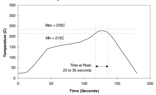
Maximum temperature slope: 5°C/second Product can withstand this profile two times.
