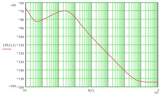
Figure 10a. Overall PLL Phase Noise (BW=5kHz)
