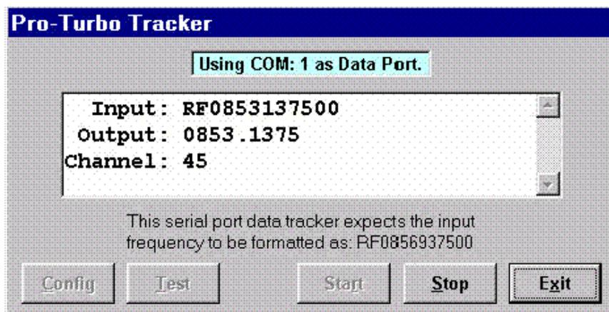
Above, the input data, decoded frequency and the channel that would be output to the scanner are shown if the trunk decoding program and data port are configured properly.
