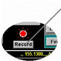
The **Record** button starts recording without a synchronised log file. The file can grow to about 36 Mega-bytes for a recording session of one hour's duration. The file is closed and a new file is created every hour. When depressed and active, the button displays the message "No Log" as a reminder.
