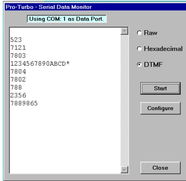
NULLs are stripped from the data flow. If a DTMF decoder circuit similar to the one included in this document is used, telephone DTMF can be decoded and displayed here and logged if desired. Any circuit that decodes DTMF and has a hexadecimal output similar to that of the MC145436 decoder should work for this monitor. The serial port used for this monitor must be a free port that is not being used by another device. It is configured similarly to the Tracker function port.
