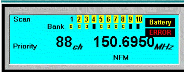
If Pro-Turbo starts and you get a screen similar to that above, your Interface has not been properly synchronised. Pressing the scanner reset switch at the rear of the scanner will correct this... OR exit Pro-Turbo and turn the scanner/interface OFF and re-start Pro-Turbo and turn the scanner/interface ON when asked by the initialisation screen.
