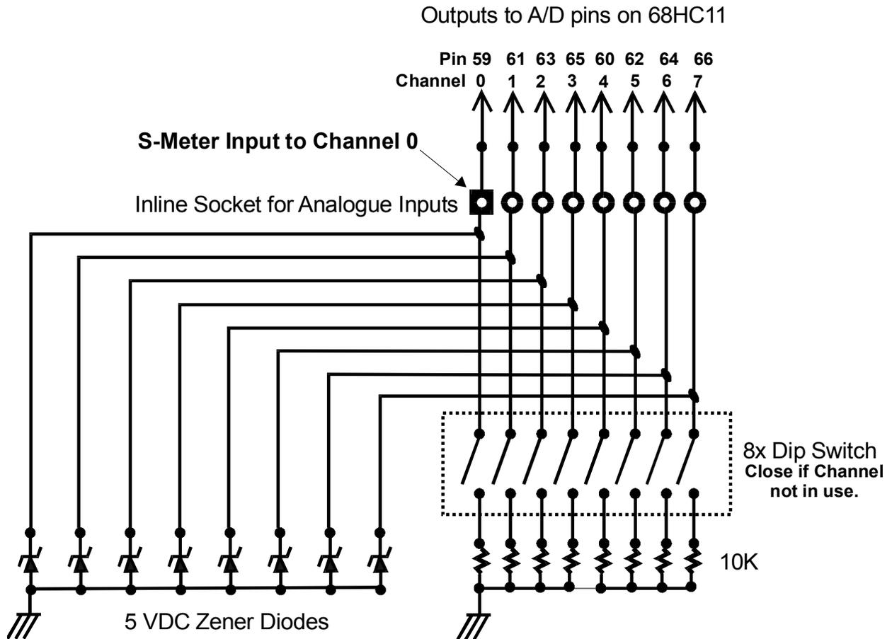
**Maximum 5VDC input allowed to A/D pins of the 68HC11**
