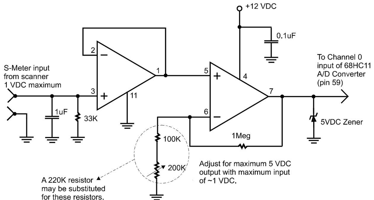
Similar circuits may be constructed to condition inputs from other devices BUT remember that the MC68HC11 A/D converters as used in the HB/CE232 interface **MUST NOT HAVE NEGATIVE VOLTAGES i.e. VOLTAGES LESS THAN 0 VDC OR POSITIVE VOLTAGES GREATER THAN 5 VDC APPLIED.**
