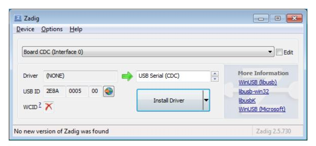
Then click Install Driver. A serial port will be assigned when the installation is complete.
