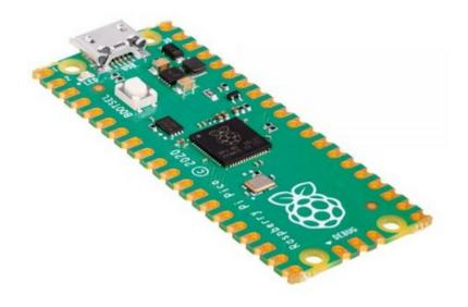
It connects to a PC using a USB cable. You will have to press the BOOTSEL button while connecting the USB socket of the PC, this opens an additional drive:
