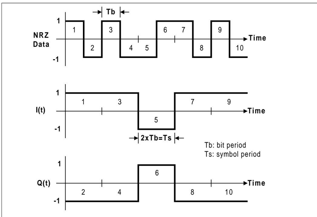
Fig.4. Serial-to-Parallel Conversion
