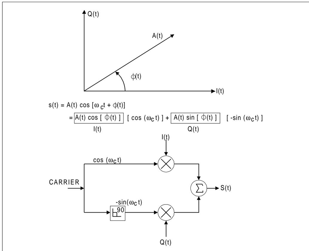
**Figure 2 - Mathematical Representation and Hardware Implementation of an I / Q Modulator**
