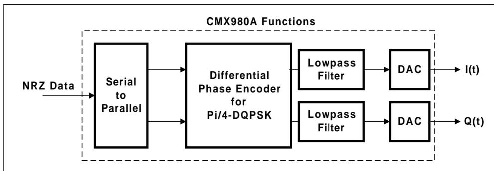
Figure 3. QPSK and  $\pi/4$ -DQPSK Baseband Generator
