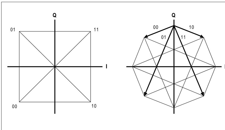
Figure 5 - Signal Constellation of QPSK and  $\pi/4$ -DQPSK
