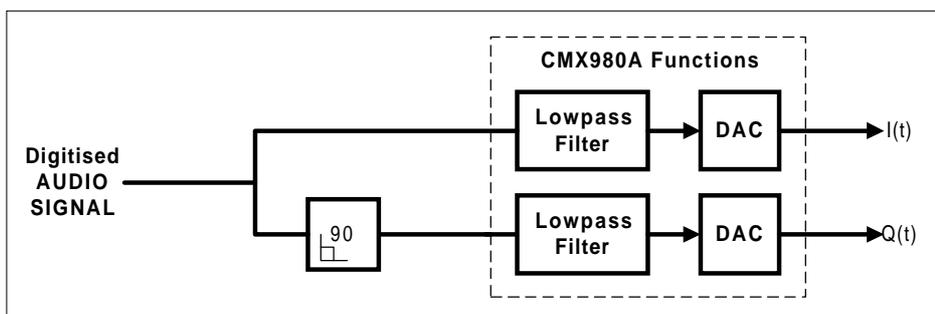
Figure 8 - Baseband Processing for SSB-AM
