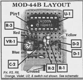
is to put a voltmeter (+) on Pin 2 of U-1 and (-) to ground and tune the scanner to a cellular or trunked data channel. Adjust VR-1, first one way and then the other and then to a point so that the voltage on Pin 2 of U-1 just becomes stable with a nice and steady +5 volts. It takes a steady +5 volts for about one second to trigger the SCAN/SEARCH RESUME function, but don't adjust VR-1 any further than necessary to stabilize the DATA/TONE voltage at Pin 2.
