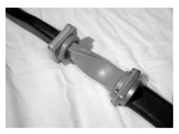
Getting waveguide to go around a rotator, or even to be flexible going up a portable mast, can be fun.
