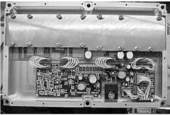
Power supply requirement is 12.6VDC @ 15amps after readjusting gain and bias.
