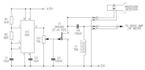
I hope this little circuit is of interest. The principle is simple and similar to that used in many sensitive RF voltmeters such as my old valve Boonton which uses an electromechanical chopper (Synchroverter) arrangement. I don't think this idea has been shown in this application before but would appreciate any references.
