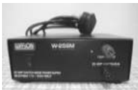
Watson PSU: 13.8V @25Apeak, 22A continuous
