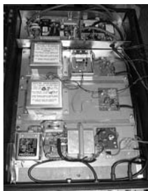
Right: The two beacons mounted on a common base plate... oscillator and PSU sections only.. these appear to be kept remote from the mast head ODU units shown on the next two photos
