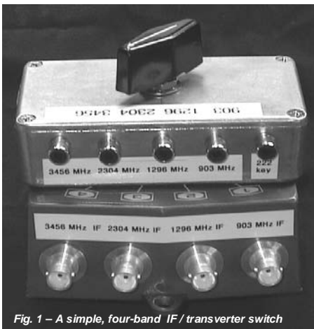
Fig. 1 – A simple, four-band IF / transverter switch
