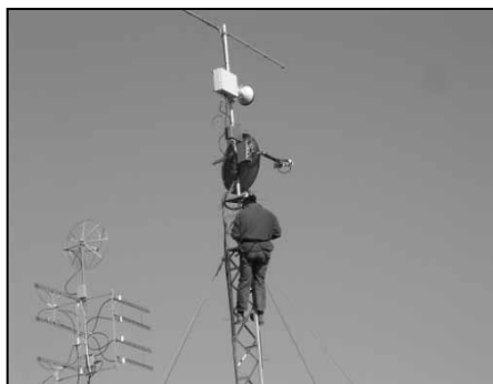
Photo: Dave, G1OGY, atop one of the 10M high masts at M1CRO/p. The stub mast has a 144MHz 9ele F9FT at the top, 24GHz transverter with horn, and a 90cm dual feed dish for 3cm and 6cm.
