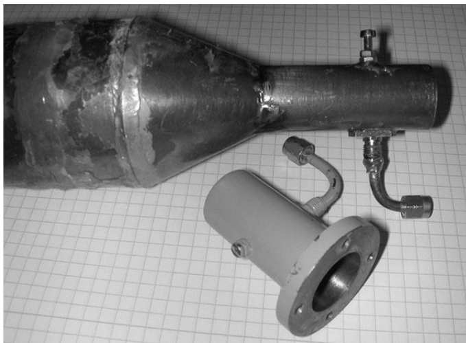
Fig. 1 Two transitions: one with a flange used on the Skobelev dual-mode feed, and the one it replaced, integrated with the old W2IMU feed.
