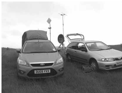
General view: Shows G8VZT 10GHz dish on tripod (before disaster!), 23cm antenna (38 ele from Severnside ATV group), plus elliptical TX horn and RX squarial for QRPP 3cm (G3UKV).
