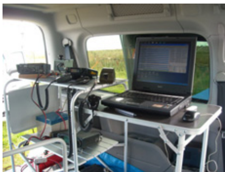
Above: G3PHO/P's operating position inside the VW Caddy Maxi Life. The fold up camp kitchen makes an ideal operating desk!
