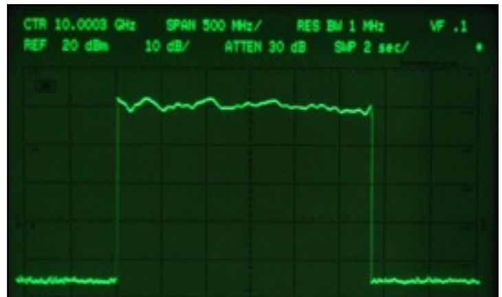
Fig 4 : The sweeper's full span (about 3GHz) showing the output amplitude flatness across that band.
