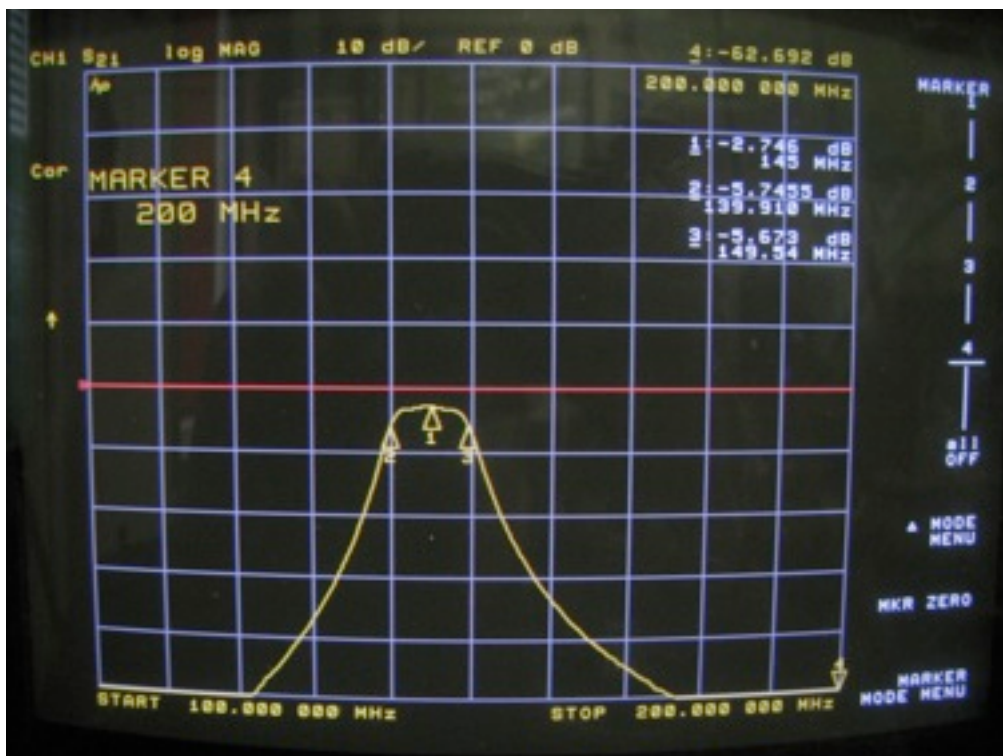
Fig 2 – Frequency response of the Chebyshev filter at a centre frequency of 145MHz
