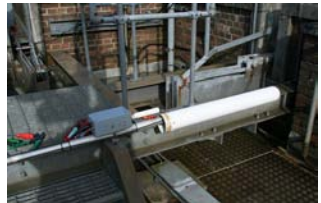
10GHz with radome with 24GHz unit (small white antenna on grey box)
