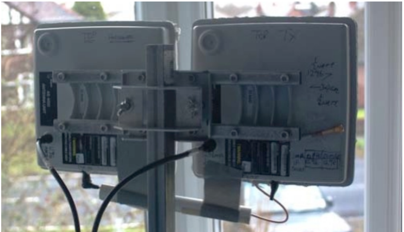
Dave G4MVU's two modified AS4000 units mounted on an old photographic tripod and position them in the front bedroom bay window
