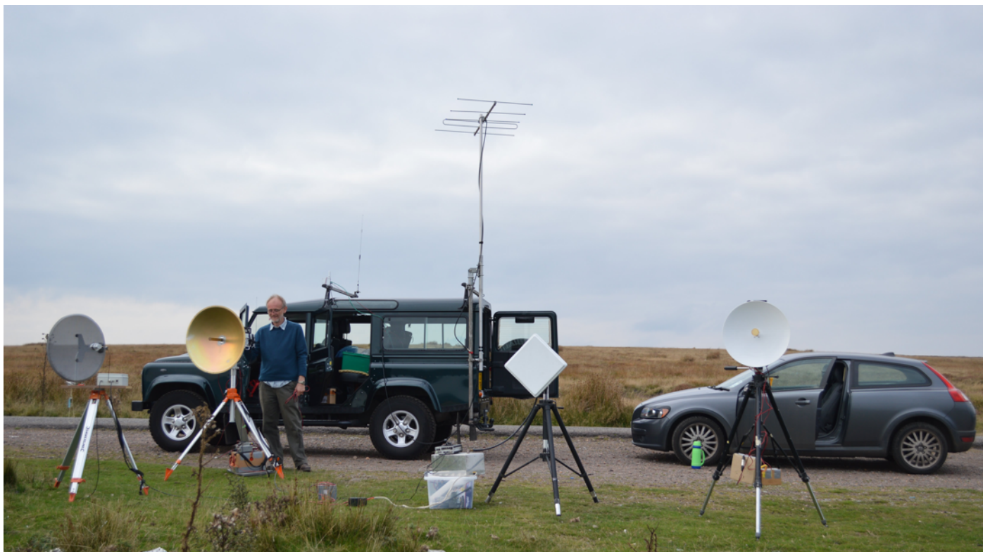
Above picture showing (L to R): 10GHz 200mW, 10GHz 10W, 5.7GHz 10W, 24GHz 500mW.
