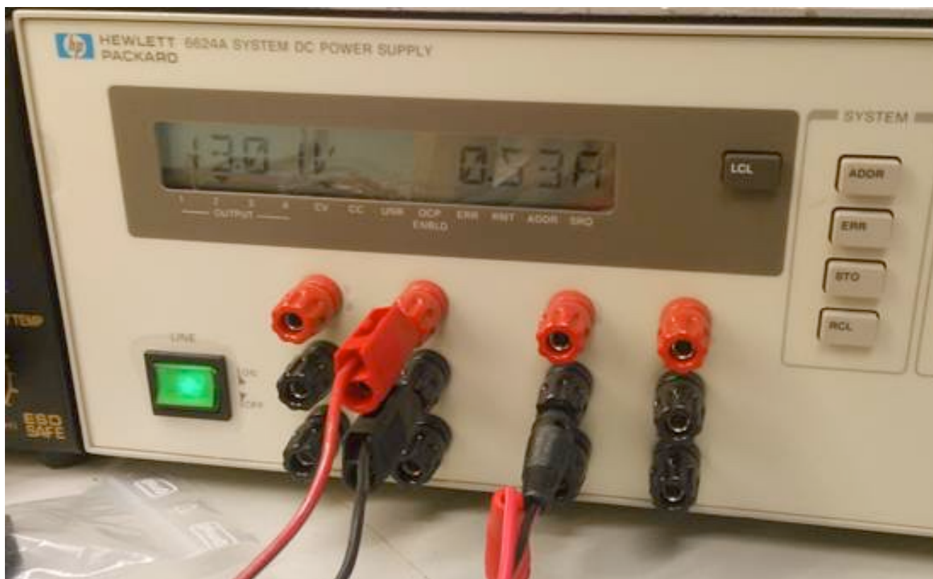
Fig.4. The amplifier under test was biased in class A with V_{\text{drain}}=13\text{V} and I_{\text{dqs}}=0.53\text{A} .
