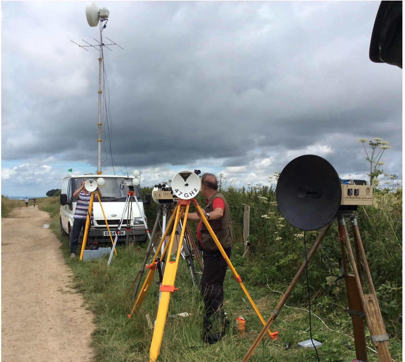
The multi-dish, multi-band set up of Chris G0FDZ/P and G8CUB/P on Hackpen Hill (Roger's 24GHz system is on the mast attached to the van).
