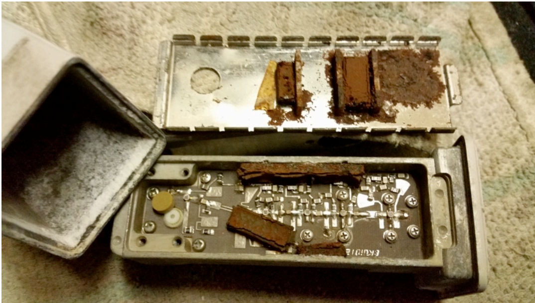
G3UVR's failed 10GHz LNA, after 25 years of service.
