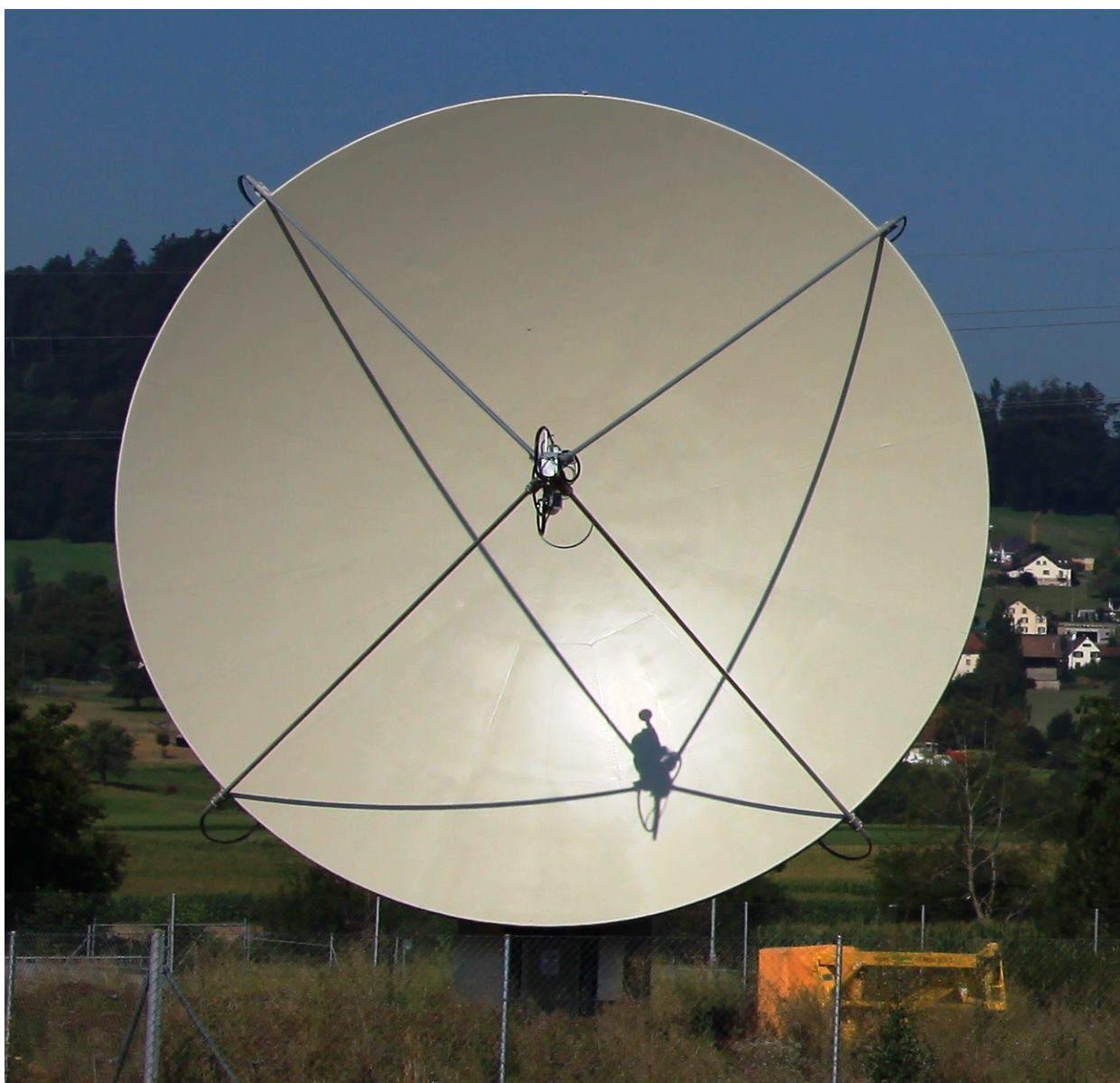
A “big gun”, the 10m solid dish of HB9Q for 23-3cm
