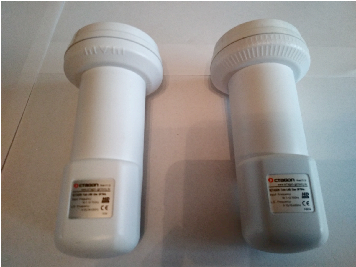
Octagon twin output LNB OTLSO types, 27MHz left, 25MHz right. Notice the skew graduations.
