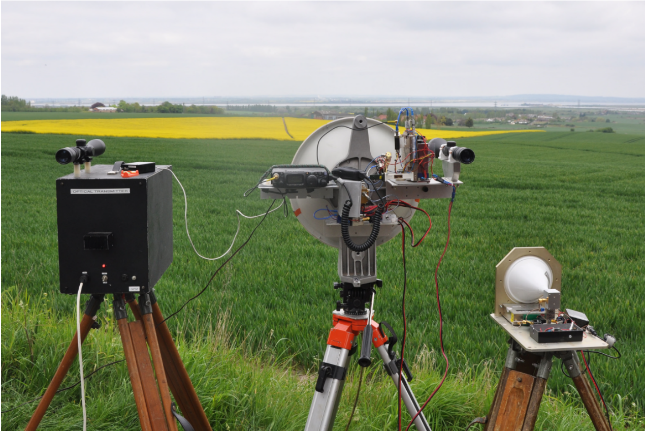
G0FDZ/P Higham LED light - 241GHz transverter with 24GHz IF – 241GHz beacon
