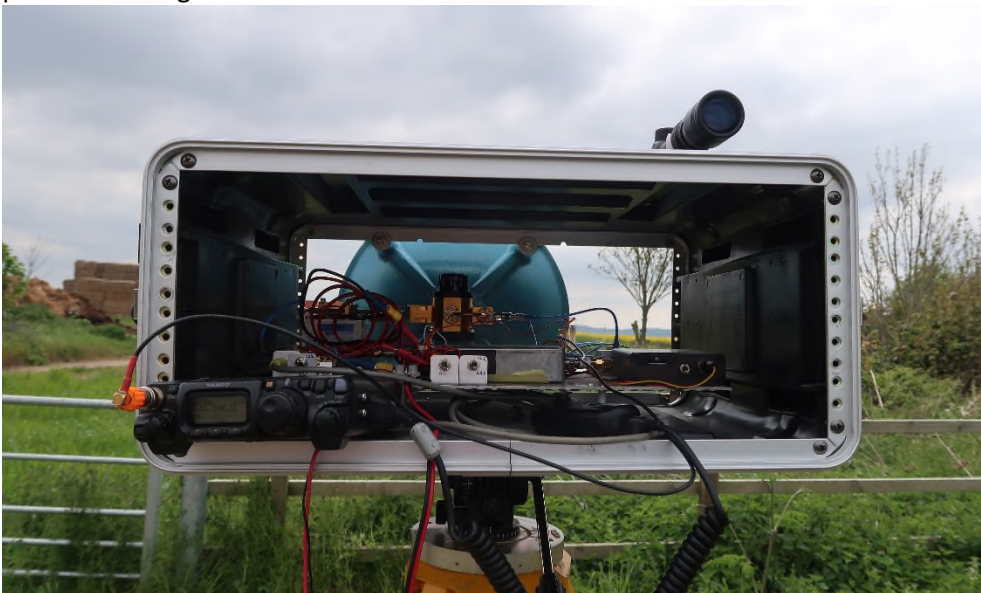
G8CUB/P West Tilbury 241GHz transverter with 432MHz IF
