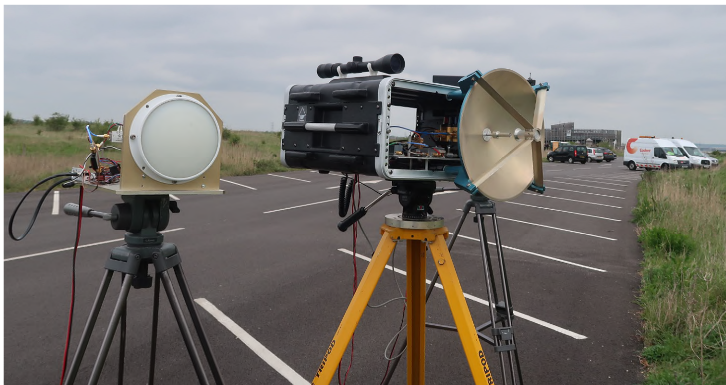
G8CUB/P Thurrock Thameside 241GHz CW beacon and 241GHz transverter
