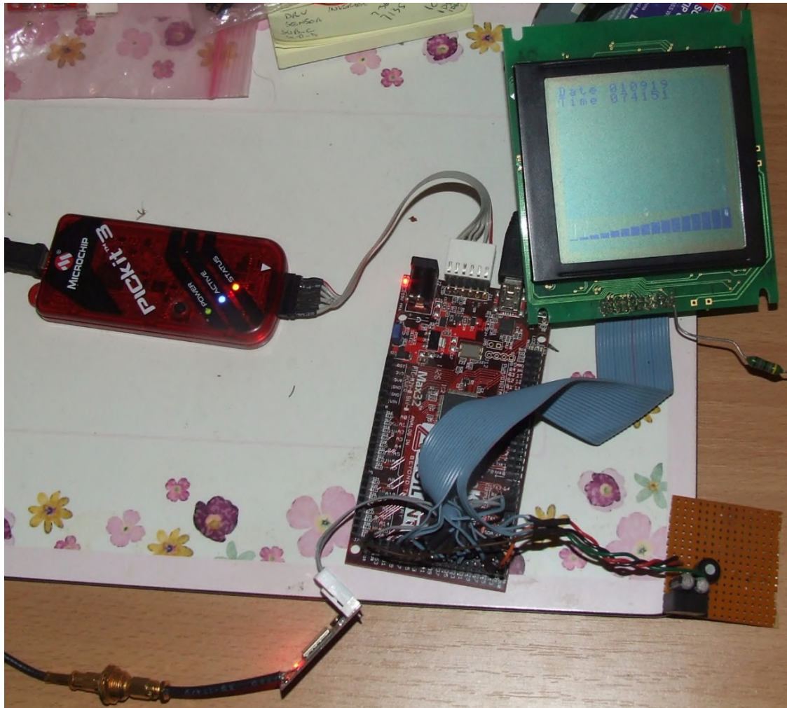
PICkit 3 in use debugging a PIC32 C/W GPS and 128 x 128 display
