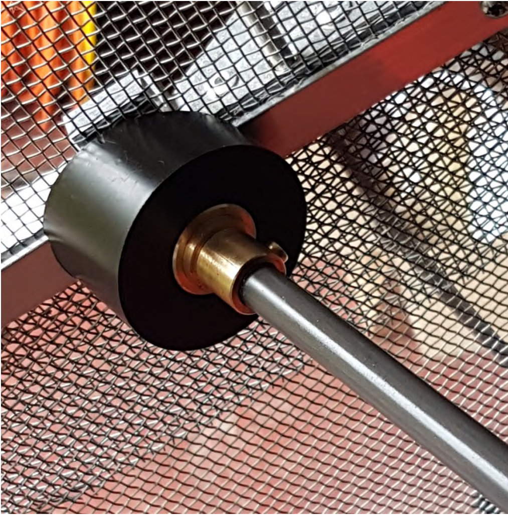
"Delrin and brass threaded socket mounted on the dish face"
