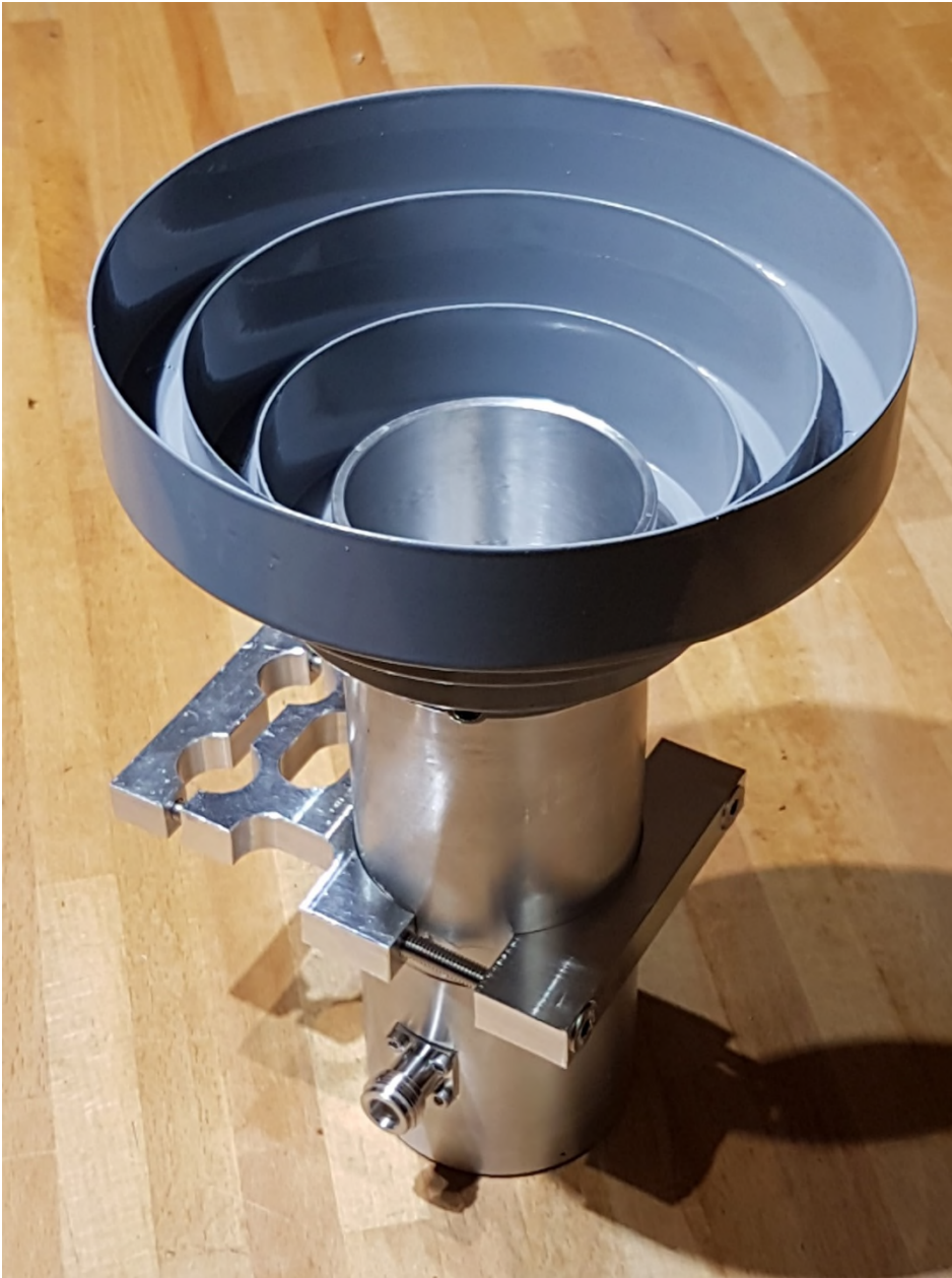
"0.71 lambda 3.4GHz feedhorn with N socket and probe"
