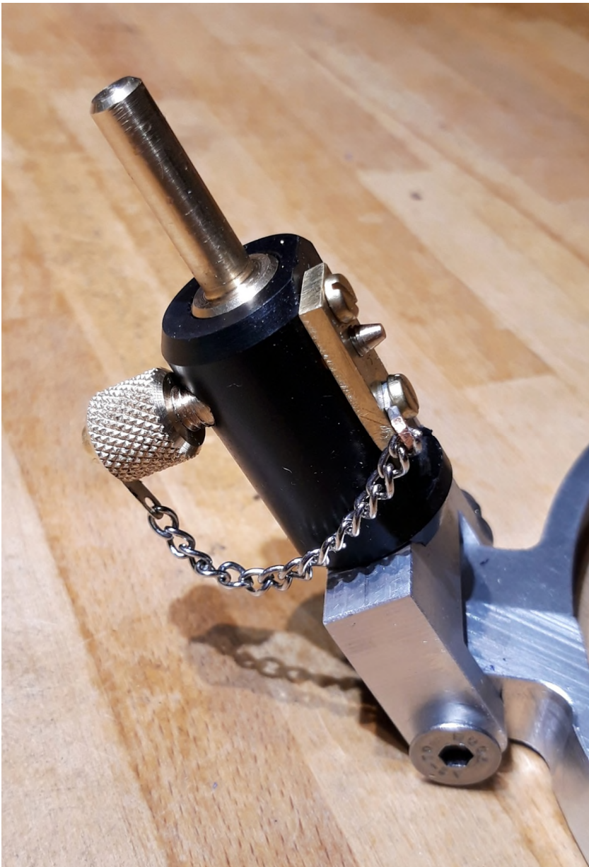
"QD socket with retaining pin in place"
