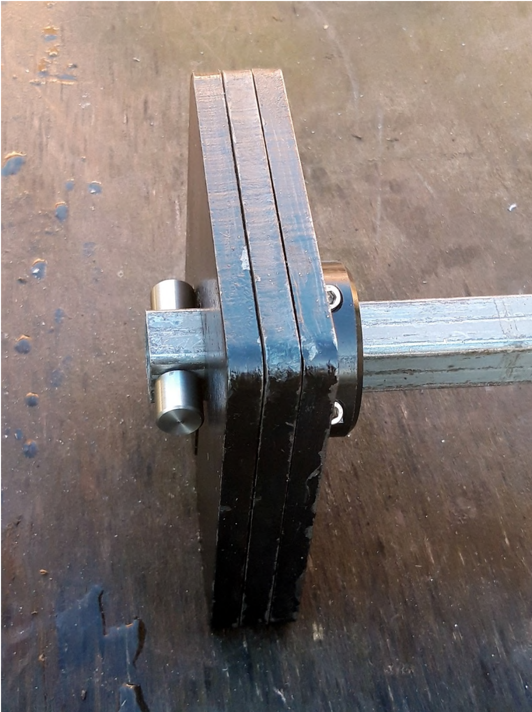
"Adjustable clamp and stainless steel end stop for the counterweights"
