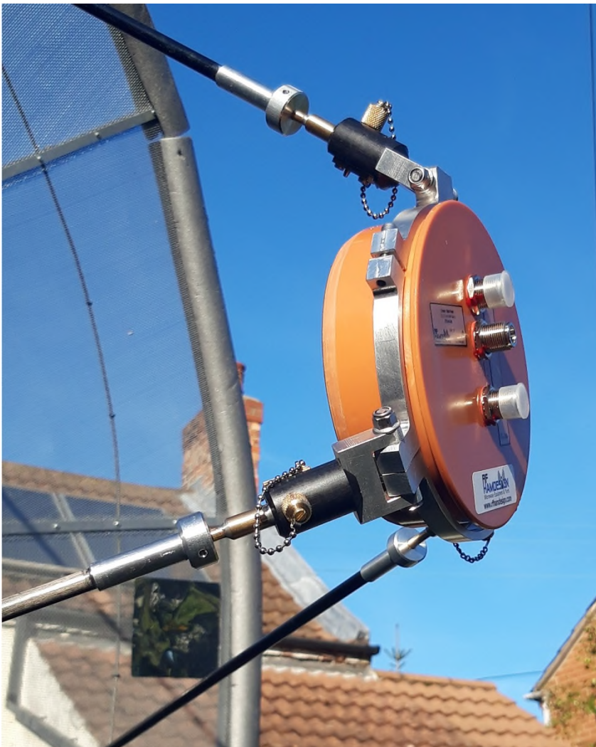
"RFHamdesign ring feed in place on the dish"
