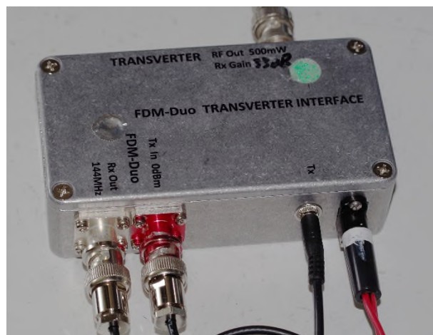
Driver Interface for the Elad FDM-Duo-Andy G4JNT
