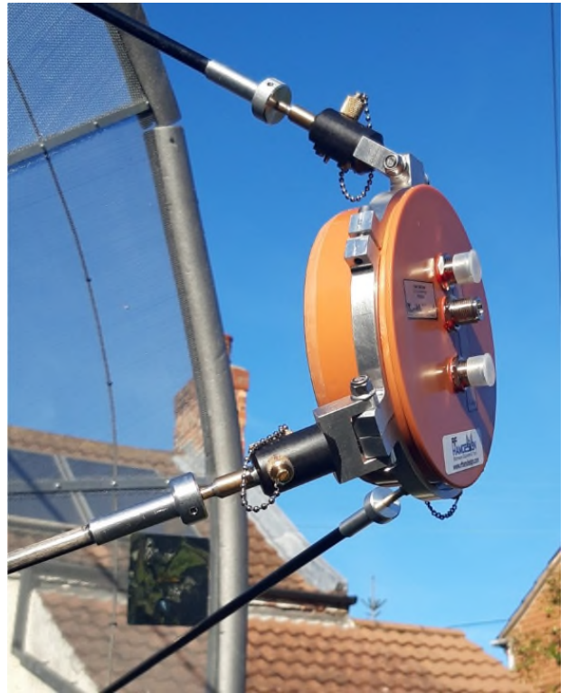
Extension block fitted into clamp ring
