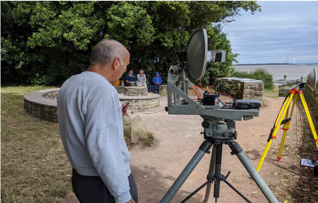
GW4LDR/P working G8GTZ/P using a non-optimised 30cm offset dish. Distance was 4.4km.
