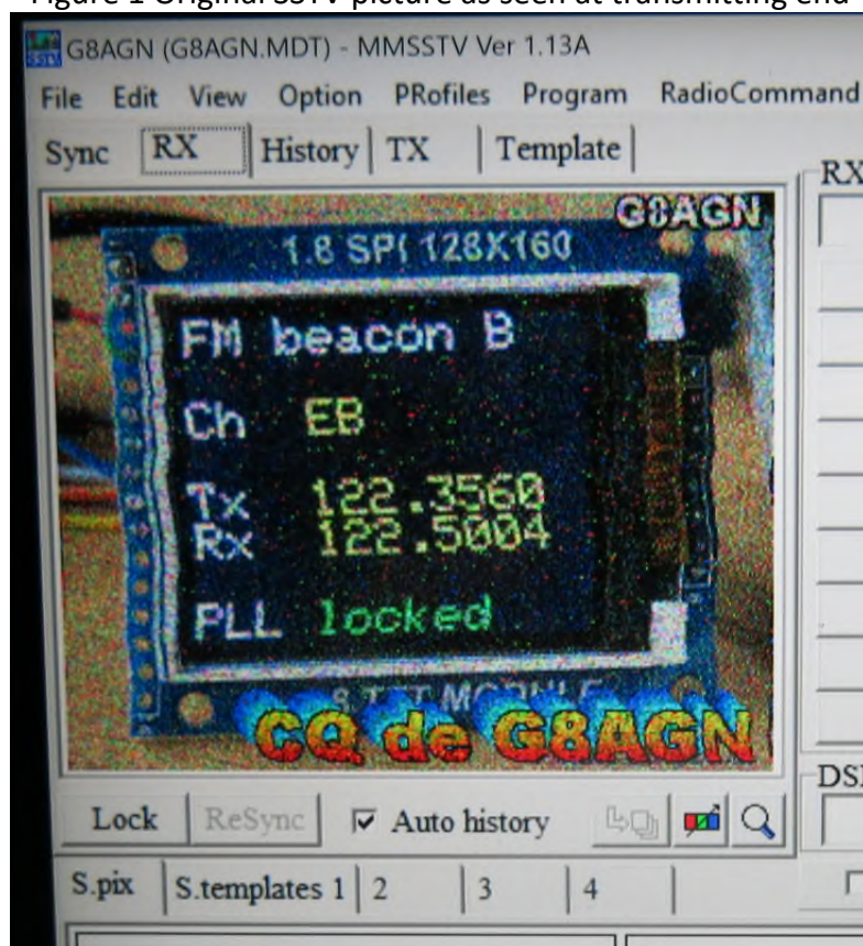
Figure 2 SSTV picture as received after transmission at 122GHz
