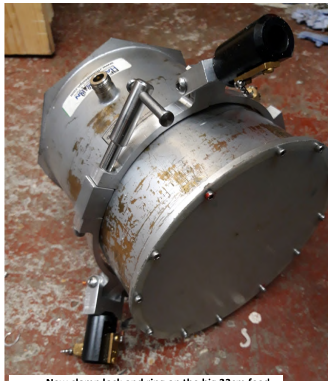
New clamp lock and ring on the big 23cm feed
