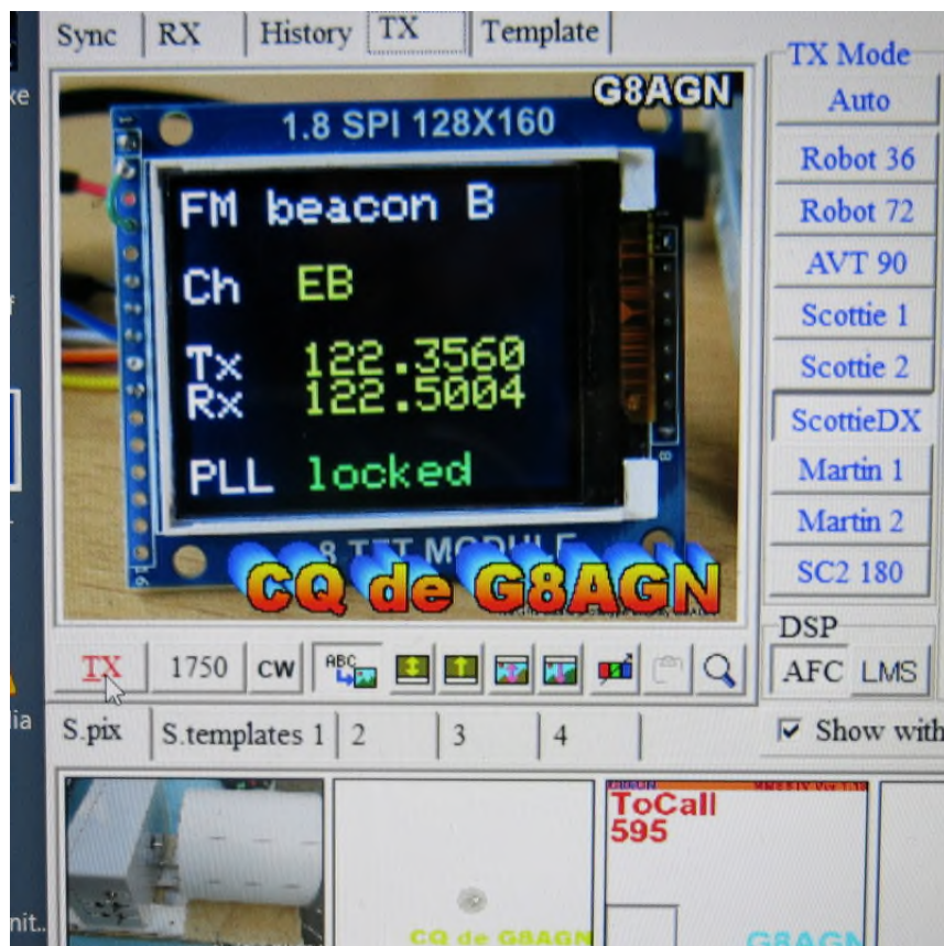
Figure 1 Original SSTV picture as seen at transmitting end
