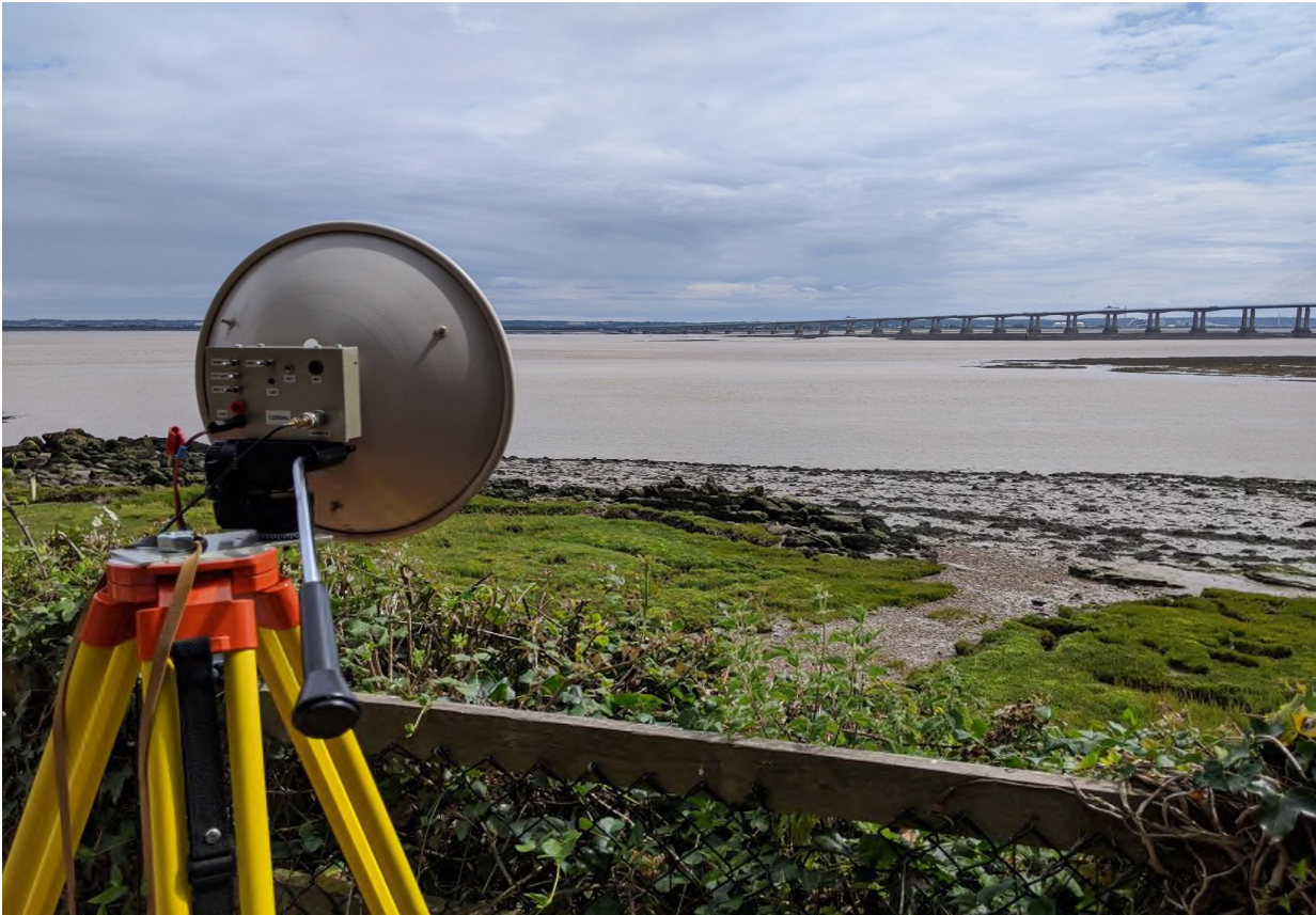
GW1EHF/P looking towards England and the new Severn crossing, a small cassegrain dish is being used.
