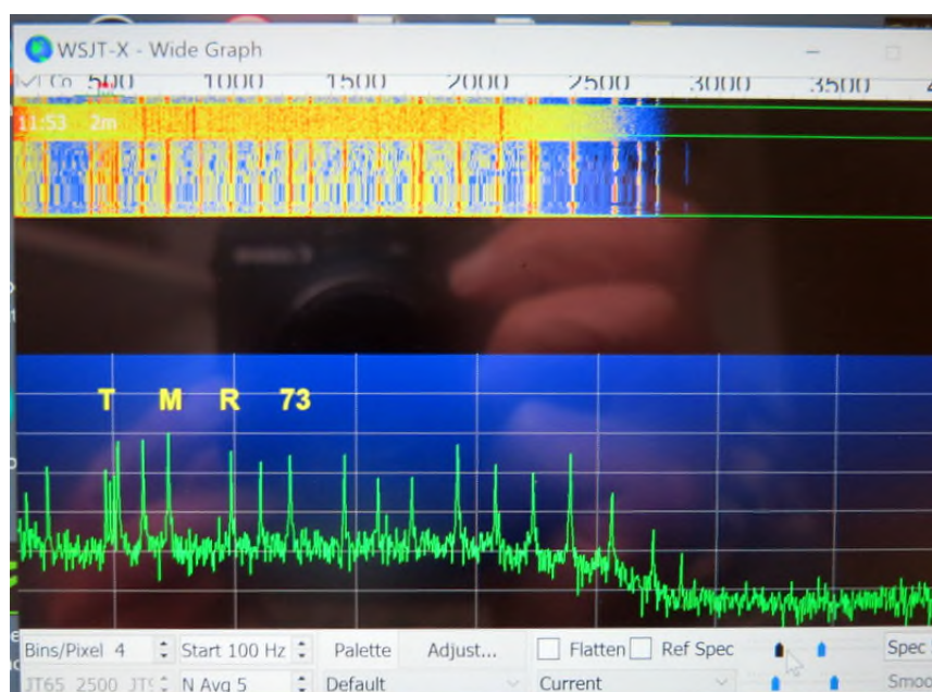
Figure 4 Spectrum of received JT4C signal from VK3CV board
