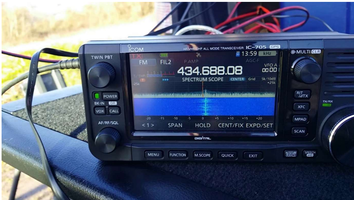
134GHz signal being received from G8CUB/P on 134GHz. That's pretty loud at 52km!
