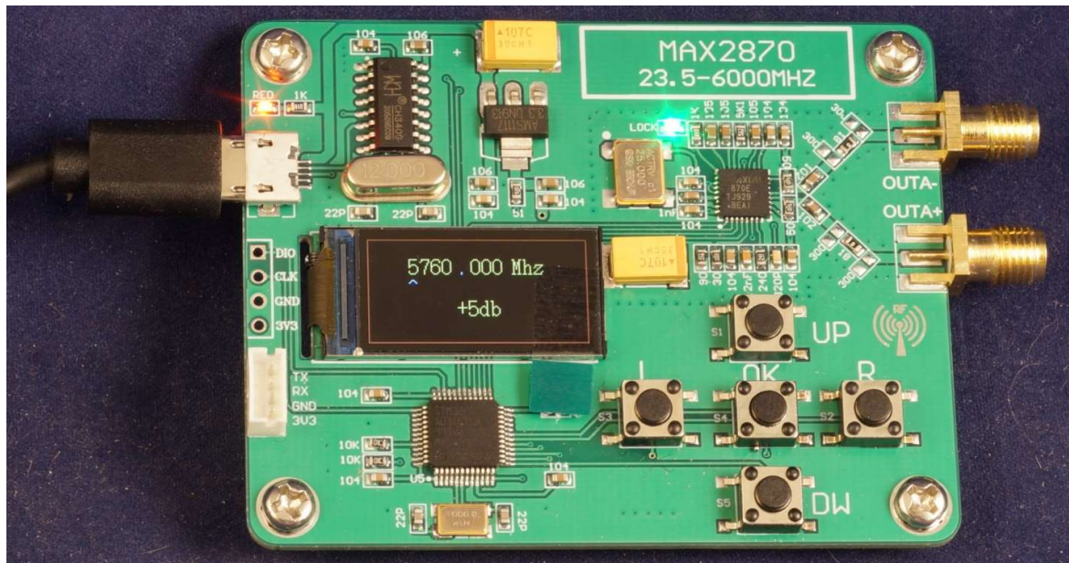
Figure new 2023 – MAX2870 Synthesizer
