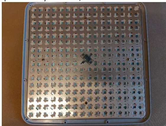
Photo 1. The 225 element array present in a Squarial
