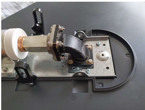
Photo 2. Waveguide interface and LNB mounting
