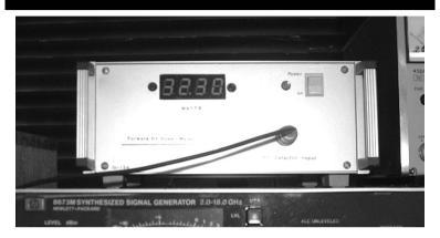
A common technique used to determine voltages at Radio Frequencies is to employ a diode detector circuit designed specifically for the frequencies and power levels of particular interest. The resulting dc voltage is proportional to the RF voltage, however this relationship is not linear due to diodes having a "Square Law Characteristic". Custom scales can be made for Analogue Panel meters but some form of linear conversion is necessary for a digital display.
