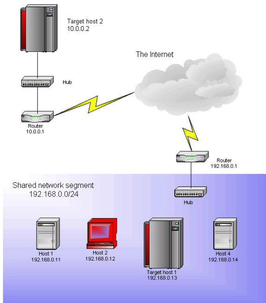
In the diagram, we have root access to host 2 and jsbach's spoofscan utility installed. Due to the fact that spoofscan sends out spoofed probe packets and then sniffs the responses using the shared network segment, we can spoof port scans from any host in the 192.168.0.\* address space launched against the target host 2 across the Internet at 10.0.0.1.
