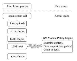
Figure 1: LSM Hook Architecture
