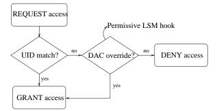
Figure 2: Permissive LSM hook. This hook allows the security policy to override a DAC restriction.
