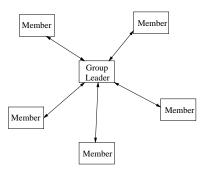
Figure 1. Centralized Enclaves Architecture
