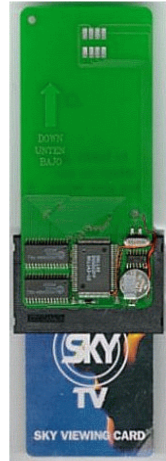
Conductive silver ink attack on BSkyB P10 card (top), with card CPU replaced by external DS5002FP (right)
