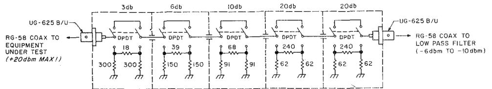
Note 1. DPDT toggle switch—Radio Shack 275-1546 or equivalent.
