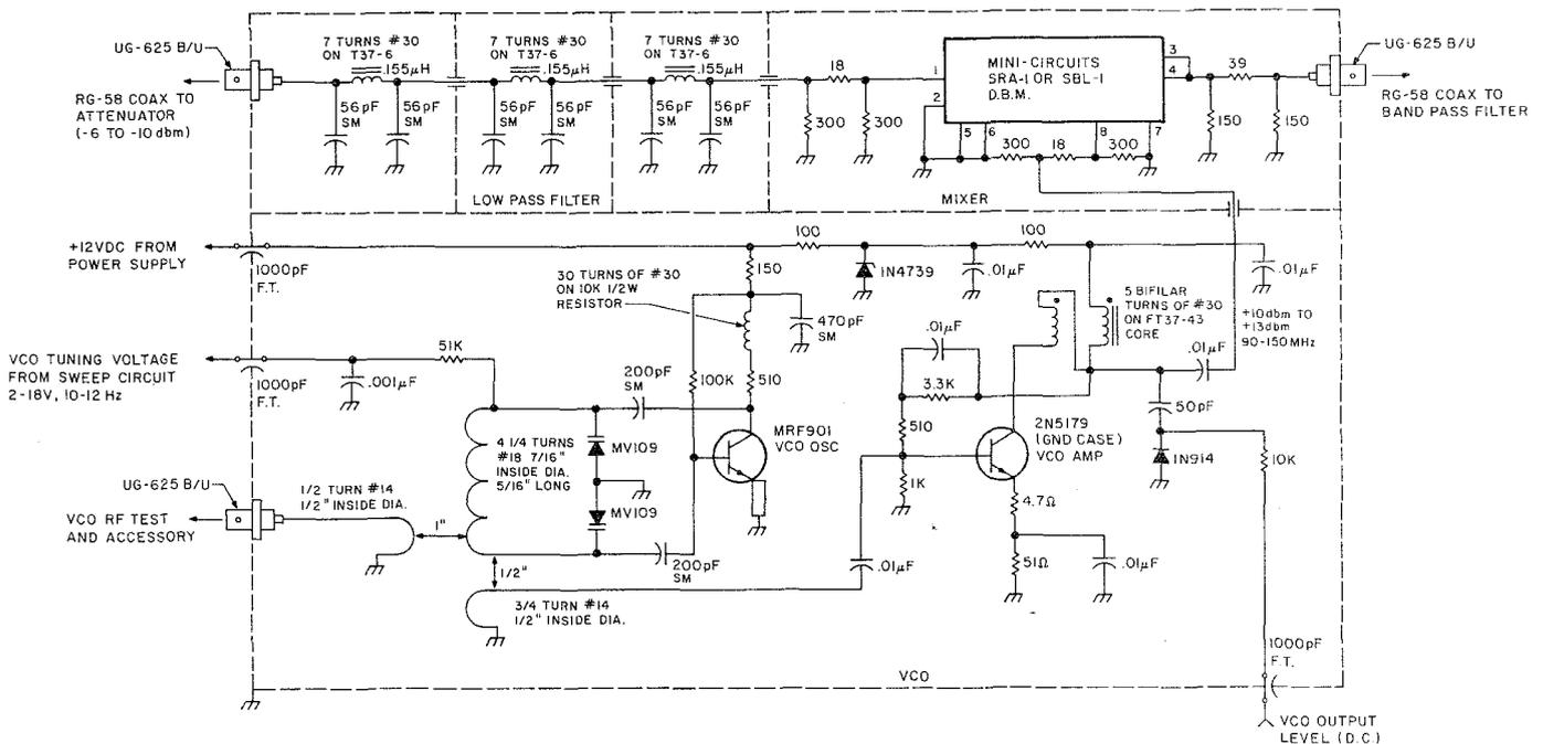
Note 1. Resistors are 1/4 W, 5%; unspecified capacitors are 50-V ceramic.
