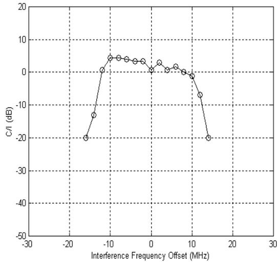
**Figure E-11** *C/I versus wideband interference frequency offset*
