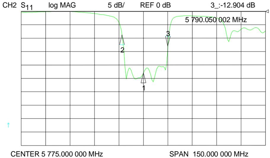
**Figure A-5 Filter with center frequency of 5.82 GHz**
