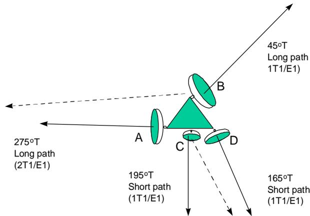
Channel assignments are first made to the longer, fading paths. With no blockage, larger antennas provide higher discriminations between the longer paths. A and D are co-channel cross-polarized; C and D are assigned an adjacent channel cross-polarized, with perhaps > 5 dB of allowable threshold degradation taken on these short nonfading hops.
