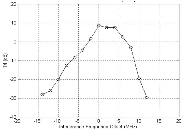
**Figure C-8** *C/I versus narrowband interference frequency offset*
