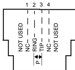
**Table 2-6 RJ-11 pinout specification**
