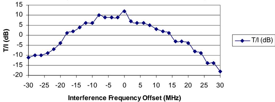
**Figure D-10** *T/I versus wideband interference frequency offset (Direction A: 05B8, Direction B: 3F0C)*
