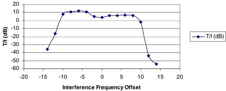
Figure D-8 C/I versus narrowband interference frequency offset
