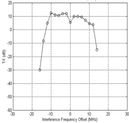
**Figure E-8** *C/I versus narrowband interference frequency offset*
