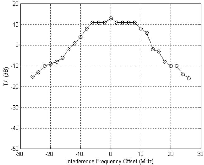
**Figure B-10** *T/I versus wideband interference frequency offset (Direction A: 1F35, Direction B: 3F0C)*
